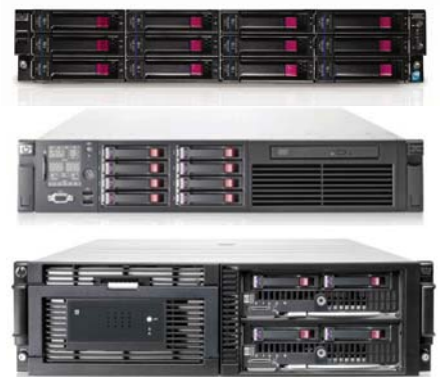
Рис. 1. Внешний вид (сверху вниз): HP X1600 G2, X3800 G2 Network Storage Gateway, X5000 G2 Network Storage System.
